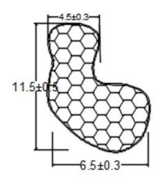
PU包覆密封条-卡槽式:KMT-M0511
