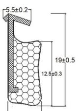
PU包覆密封条-卡槽式:KMT-C0802
