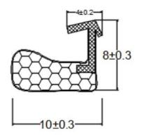
PU包覆密封条-卡槽式:KMT-C0901
